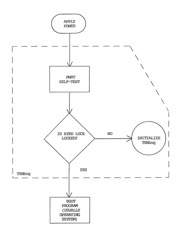
FIGURE 2-1. Flow Diagram of VME/10 Cold Start
