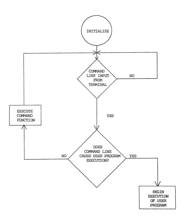
FIGURE 2-2. Flow Diagram of TENbug Operational Mode
